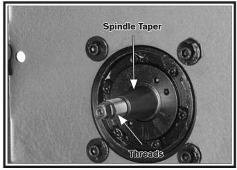
Figure 35. Spindle taper.
